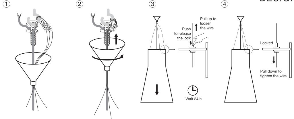
Install the power cord and support wires as illustrated.
