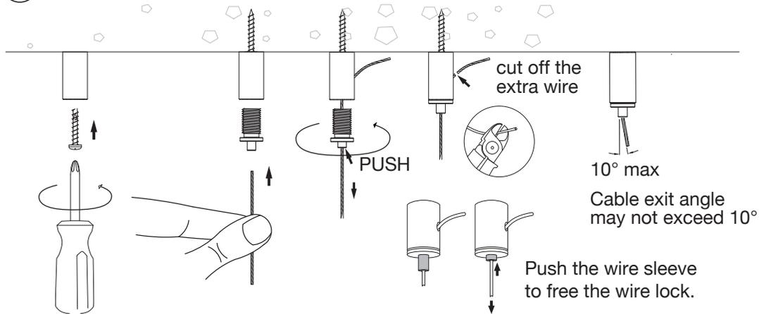
Be sure to insert the wire into the holder at least far enough to be able to clearly see it protrude from the other end of the holder. When attaching the holder into concrete or stone, use a screw anchor.
