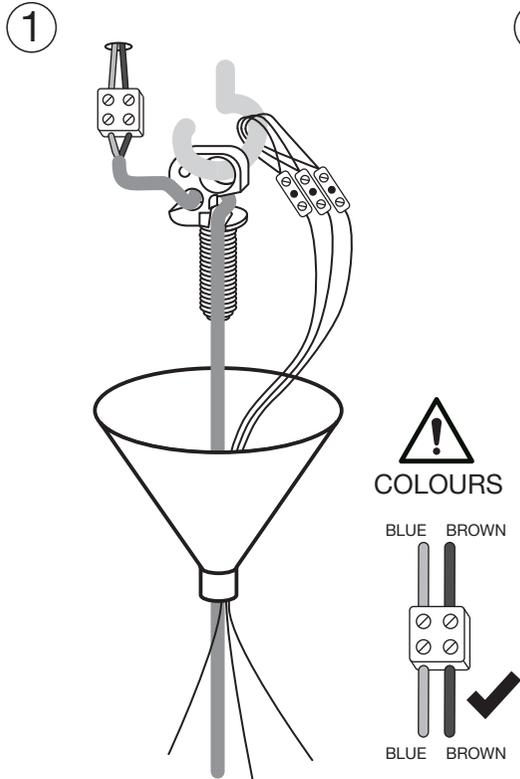
Install the power cord and support wires as illustrated.
