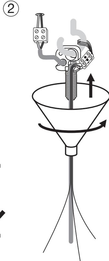
Insert the wires into the cord slot.
