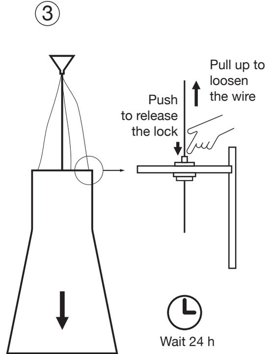
Loosen all three steel wires and let the whole weight of the lampshade rest on the power cord only.
